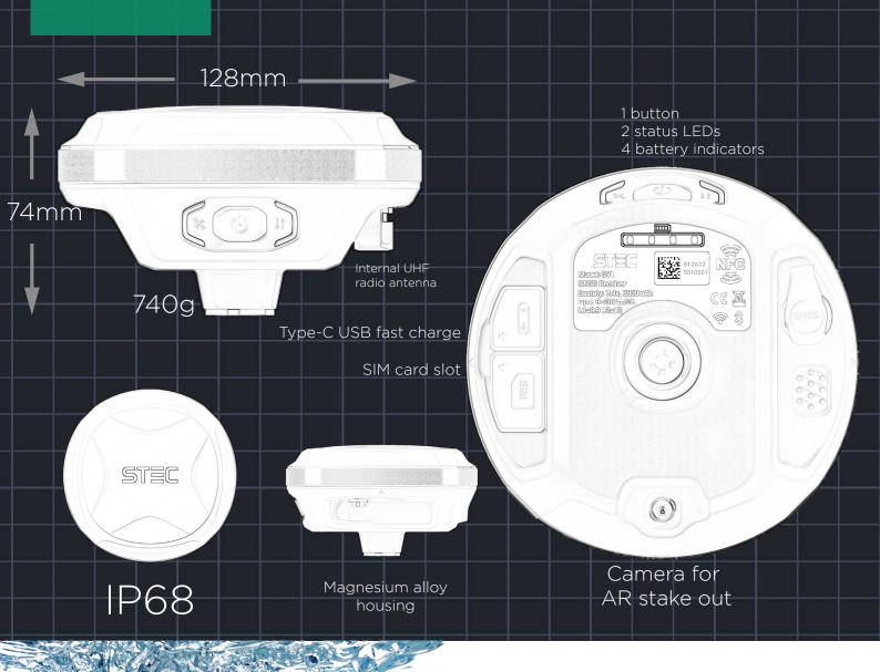
Complied with the harshest standard of IP68 water and dust proof in industry, SV1 can survive in water at 1m depth for at least 1 hour even in power-on status.
